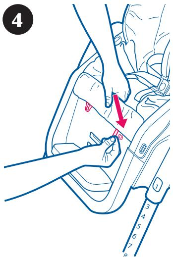
Secure the seat pad by wrapping elastic straps around bottom of seat, hooking elastic straps as shown.
